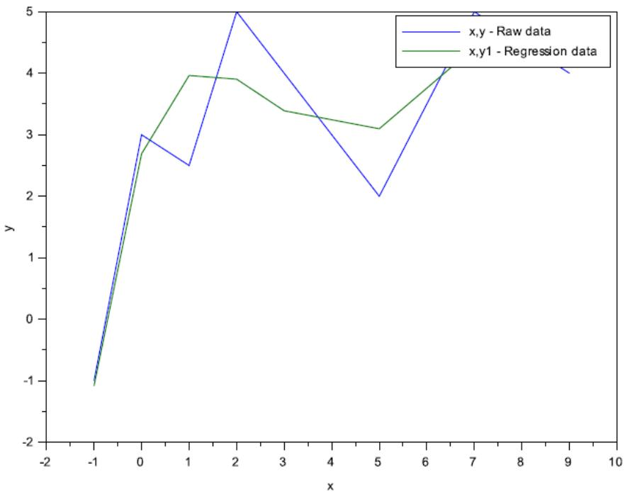
2. Fit 3<sup>rd</sup> order polynomial for the data given in problem 1. using linear regression analysis technique. Plot the data (raw x-y data before the polynomial fit and the x-y data from the regression equation) and show the graph in SCILAB.
