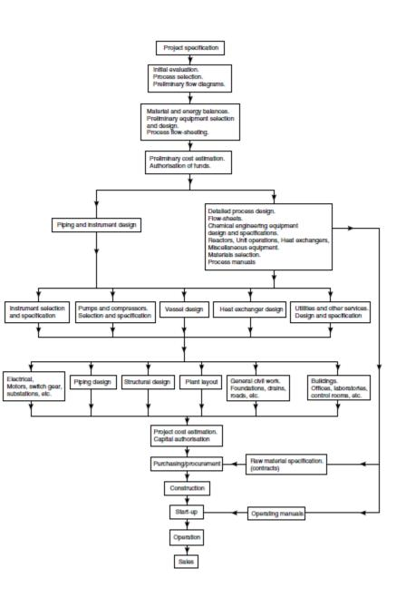
11. Draw the detailed structure of chemical engineering project representing basic and detailed engineering. **(8 Marks)**
