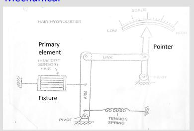
The movement made by the free end of the spring operates the instrument pointer.
