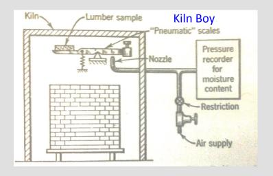
The resulting air pressure is indicated by the simple pneumatic nozzle system, and the resulting pressure is indicated at the receiver.
