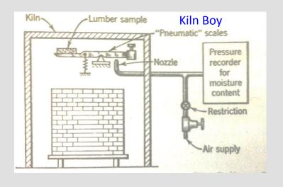
This method is used for measuring the moisture content of kiln dried lumber.
