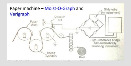
Moist-O-Graph operates by measuring the electrical resistance through the paper
