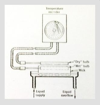
The depression of temperature of the wet bulb versus the dry bulb can be correlated with water vapor pressure using the equation
