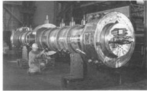
Polyethylene reactor; this 16-in inner-diameter reactor is designed to operate at 35,000 psi and 600°F; in operation, this reactor is in a vertical configuration. Courtesy of Autoclave Engineers, Division of Snap-lite, Inc.
