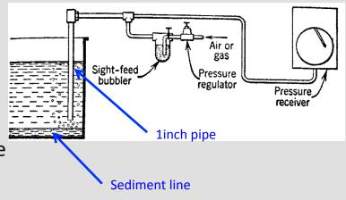
Classification based on applications – Bubbler System (Open Vessels)
