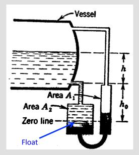
Classification based on applications – Interface level (Differential pressure manometer)
