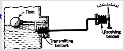
The movement of float causes a displacement of metallic bellows which is filled with oil.
